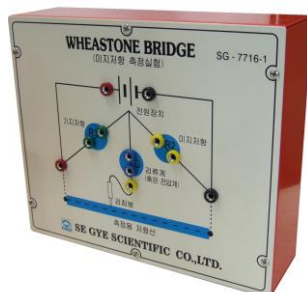
휘스톤브릿지 제어기(Wheatstone Bridge Control Box)
